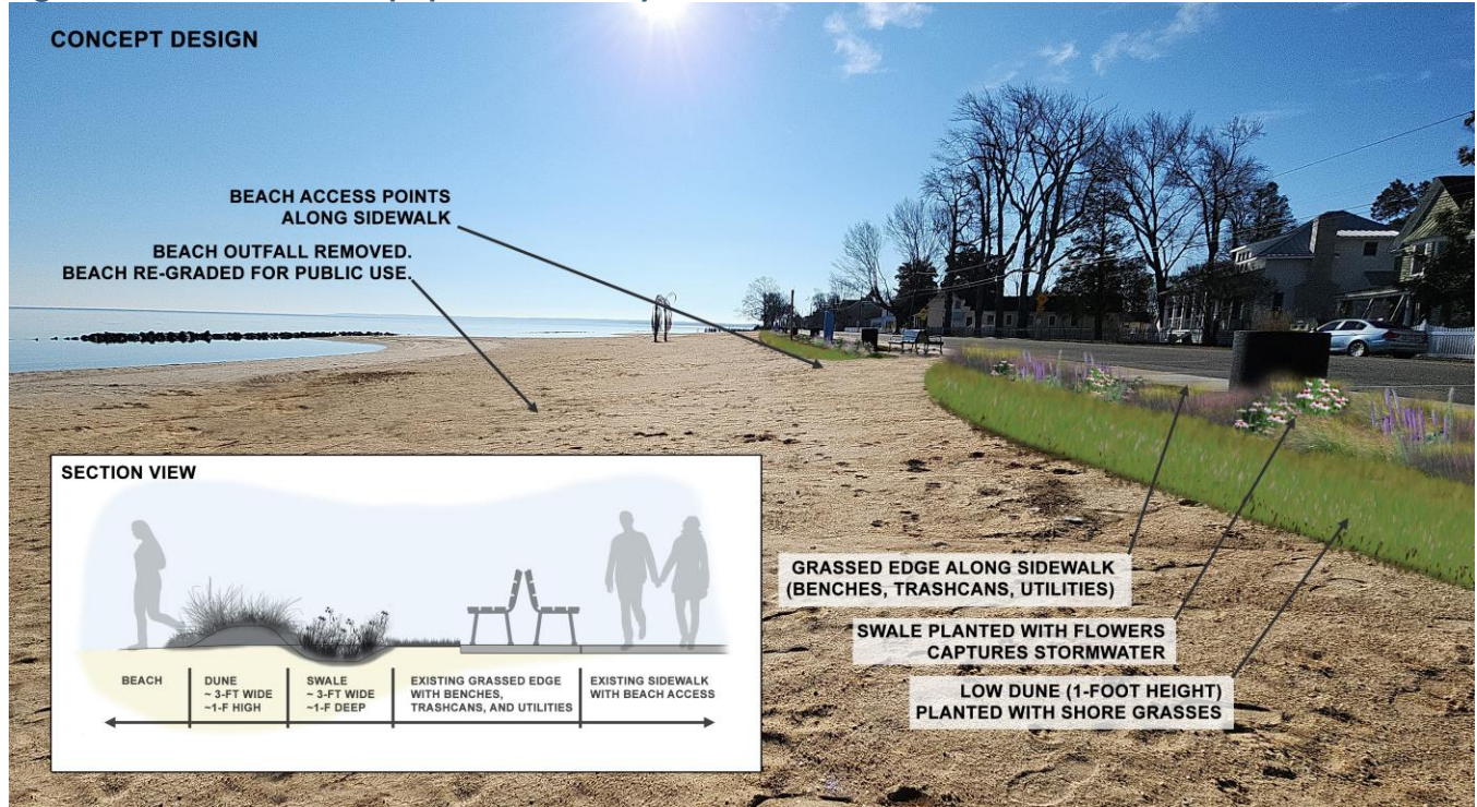
Figure 2-17: Initial concept plan for Priority Area #2: Potomac River Outfalls
